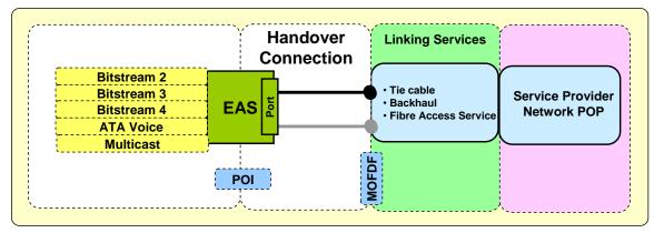
This is a generic diagram showing the standard configuration and service demarcation points. It is not intended to represent every situation or detailed physical architecture. The following point should be noted:
